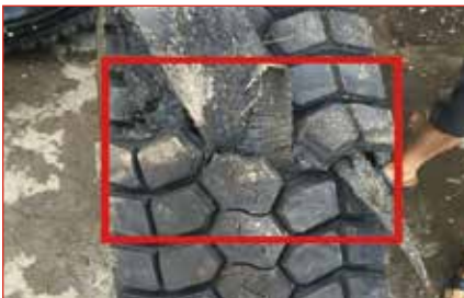
Tire Crown Impact Blast
