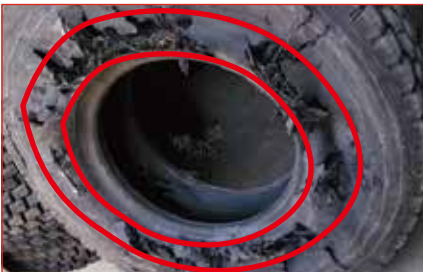
The Carcass Was Crushed By Running Without Air
