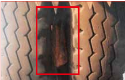
Foreign Material Between Side Wall
