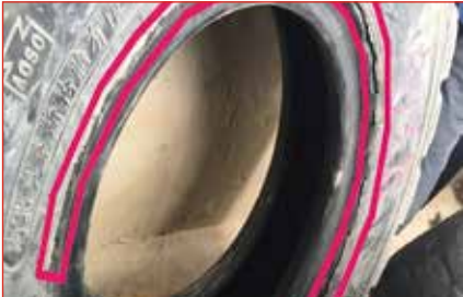
Bead Twisted And Deformed To Crack
