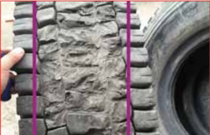
Pattern Block Cracking Or Dropping Off
